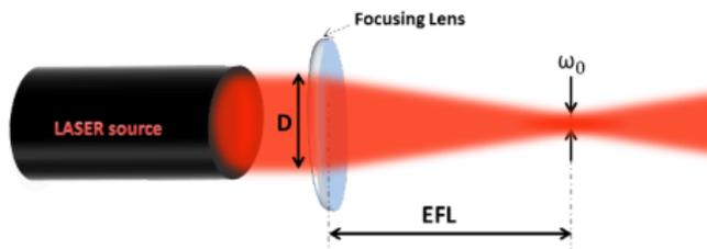
Quick estimate:  $1\mu\text{m}$  spot size  $\sim 4 \times 10^6$  unit cells of Si ( $a \sim 5\text{\AA}$ ).
