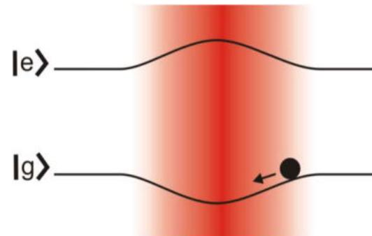
Single Beam Dipole Trap
