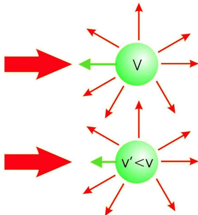
Laser Cooling, Preparation, and Readout
