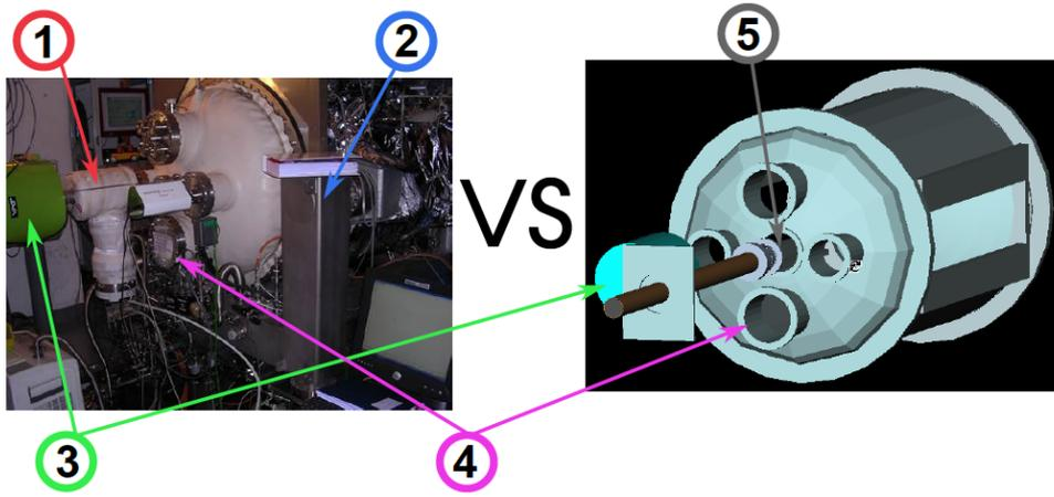
Material in front of MoEDAL detectors mapped into Geant4 simulation
