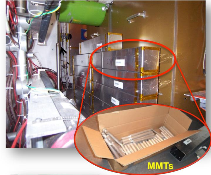
11 boxes each containing 18 aluminium rods of 60 cm length and 2.54 cm diameter
