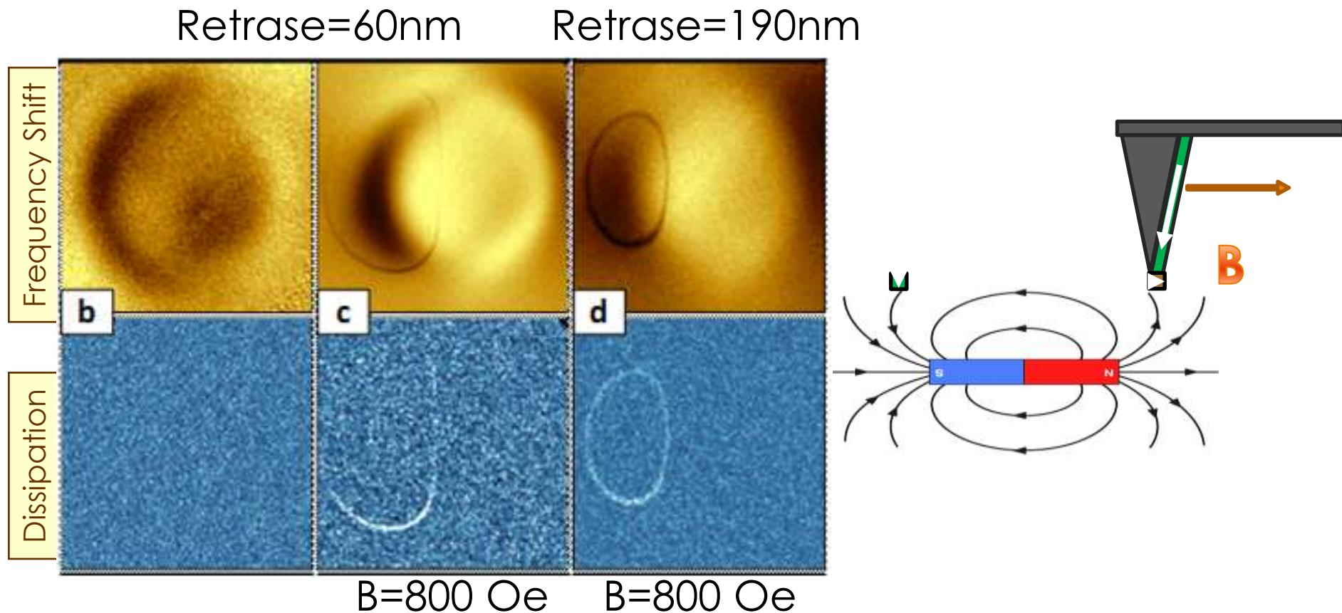
A ring appears in one side when the **Py dot is saturated** under in-plane magnetic field.
