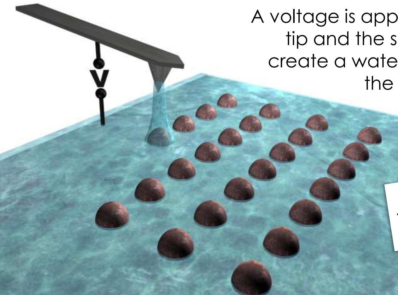
A voltage is applied between the tip and the sample in order to create a water meniscus where the oxidation occurs.
