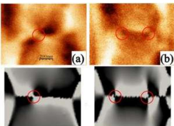
High resolution MFM images (up) and results of micromagnetic simulation (down) for vortex (a) and double vortex (b) DWs in nanostripe
