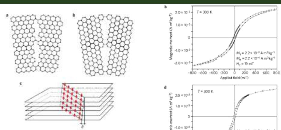
Figure 4 | Schematic models of two basic shapes of grain boundaries in graphite. a: Armchair direction with periodicity. b: Zigzag direction with
