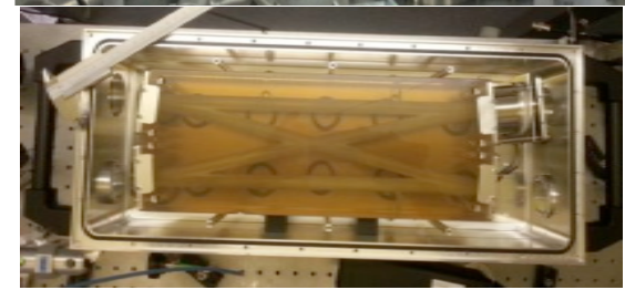
The 100W amplifier on the laser bench
