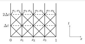
WB scheme, N = 4. The segments with speed 0,  $\pm 1$  correspond to the location of the discontinuities.
