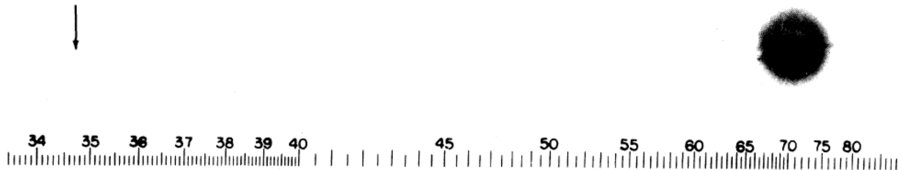
FIG. 1. A direct reproduction of the first plate in which there was an indication of second harmonic. The wavelength scale is in units of 100 A. The arrow at 3472 A indicates the small but dense image produced by the second harmonic. The image of the primary beam at 6943 A is very large due to halation.
