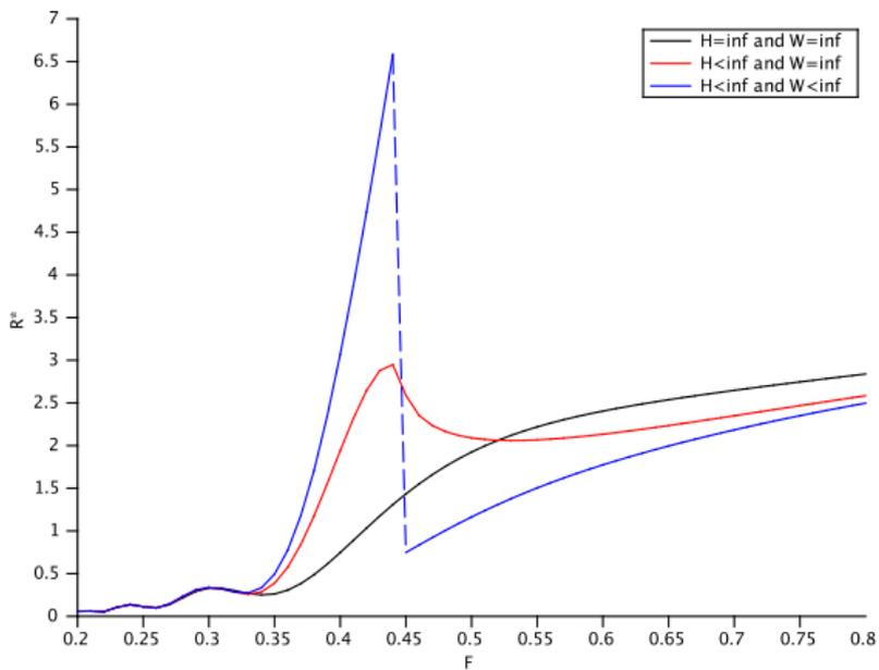
Wave resistance of a Wigley hull for 3 different domains
