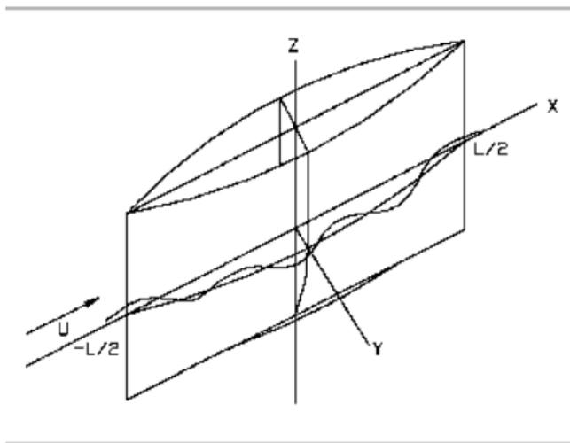
Consider a ship moving with constant velocity  $U$  on the surface of an unbounded fluid.
