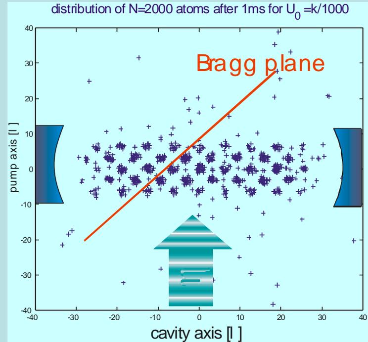
*Atoms order in regular tube-lattice structure with Bragg planes optimizing scattering to the cavity*
