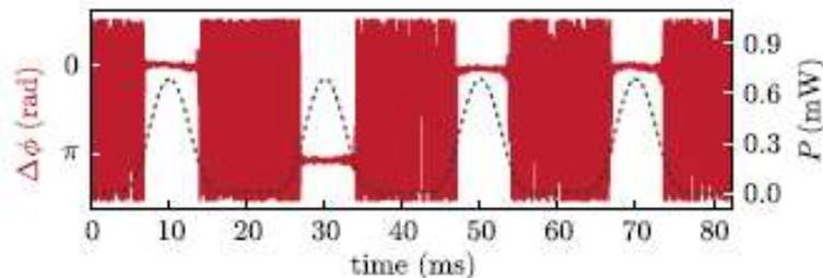
FIG. 34 (color online). Observation of symmetry breaking at the self-organization transition with a BEC. The relative pump-cavity phase  $\Delta\phi$  monitored on a heterodyne detector while repeatedly entering the self-organized phase by tuning the transverse pump power  $P$  (dashed) is shown. The system organizes into one out of two possible checkerboard patterns corresponding to the two observed phase values differing by  $\pi$ . From [Baumann \*et al.\*, 2010](#).
