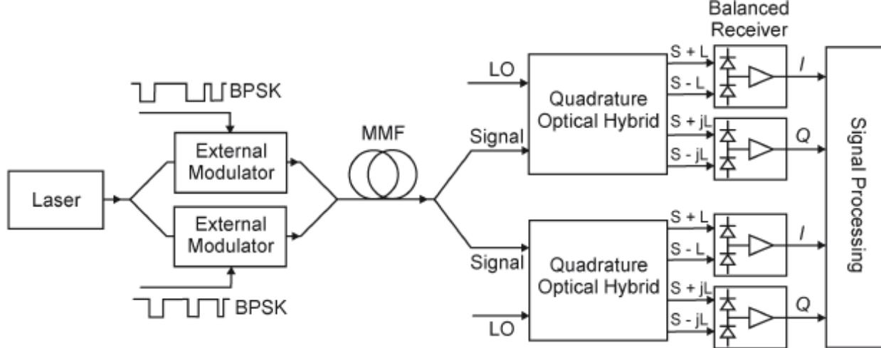
Fig. 2. Block diagram of COMIMO showing two independently modulated carriers and two receivers. Coupling diversity is not shown for simplicity.
