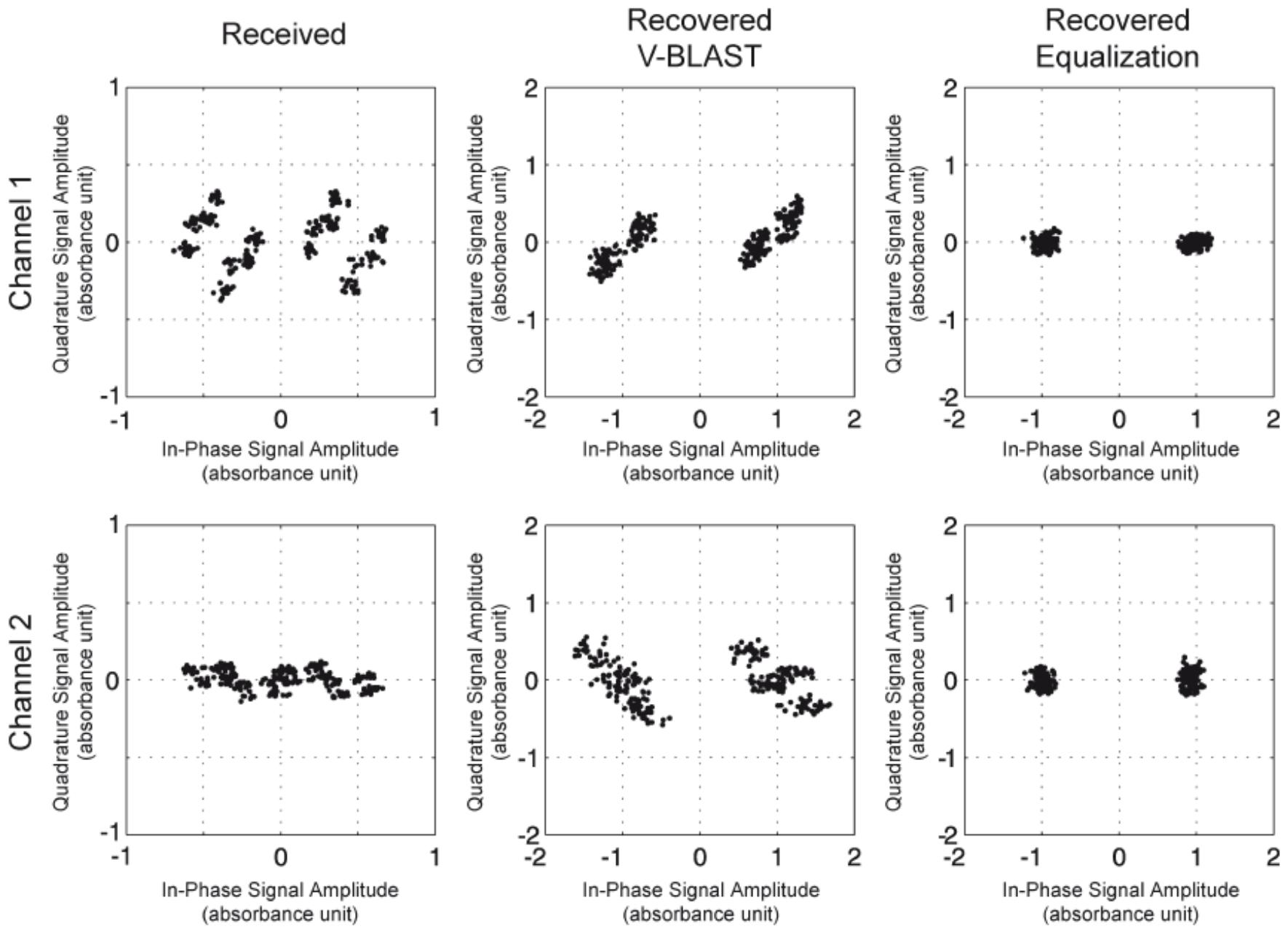
Fig. 5. Constellation diagrams showing received data from a wide-band channel (with ISI) and symbol recovery without equalization and with equalization.
