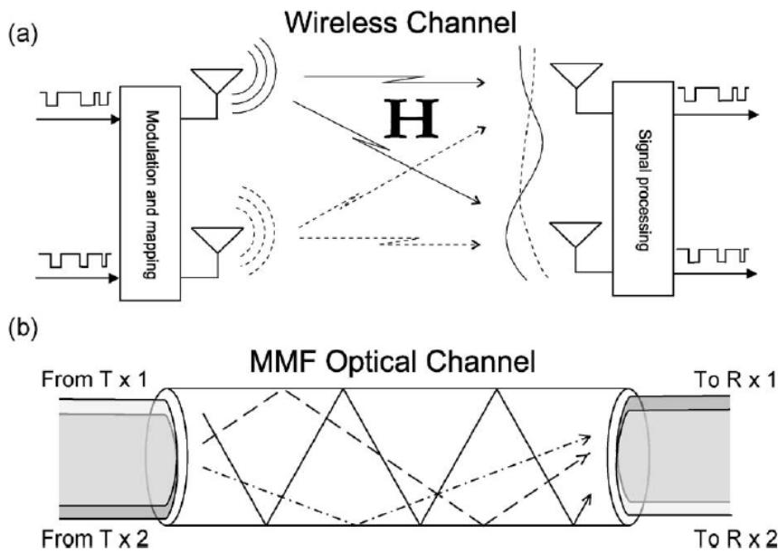
Fig. 1. (a) Coupling diversity into and out of MMF. (b) Ray tracing conceptual description of light beam scattering inside a multimode fiber.
