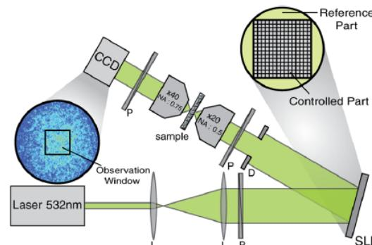
FIG. 1 (color online). Schematic of the apparatus. The laser is expanded and reflected off a SLM. The phase-modulated beam is focused on the multiple-scattering sample and the output intensity speckle pattern is imaged by a CCD camera: lens (L), polarizer (P), diaphragm (D).
