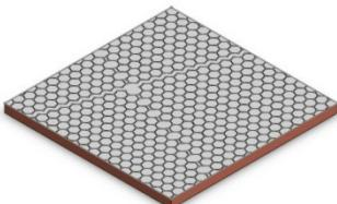
Graphene layer growth by CVD on a copper substrate
