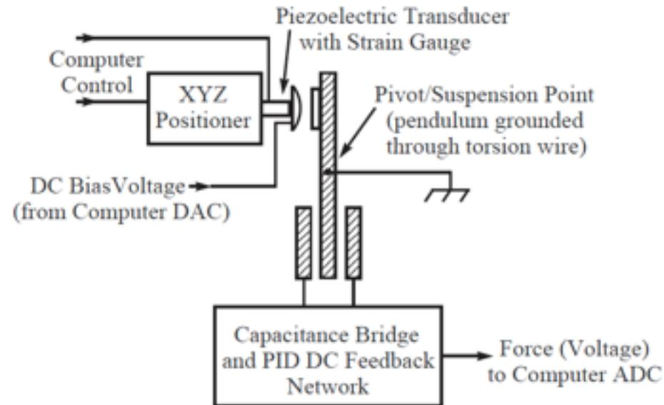
A proportional integro-differential (PID) controller provides a feedback correction voltage  $S_{\text{PID}}(d, V_a)$  to the compensator plates, restoring equilibrium.
