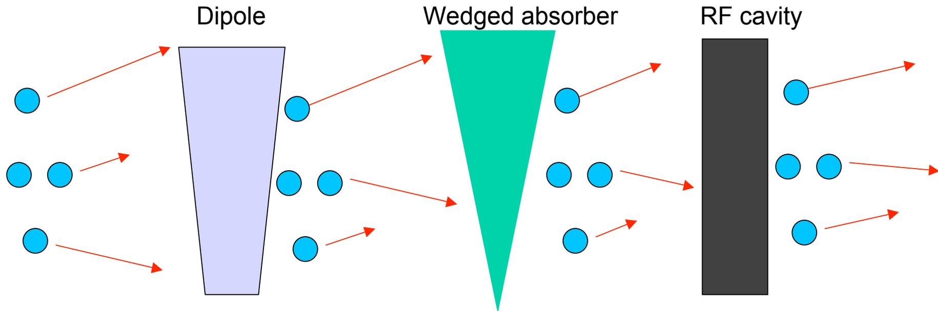
Dispersive elements (dipoles) and wedged absorbers allow also longitudinal cooling.
