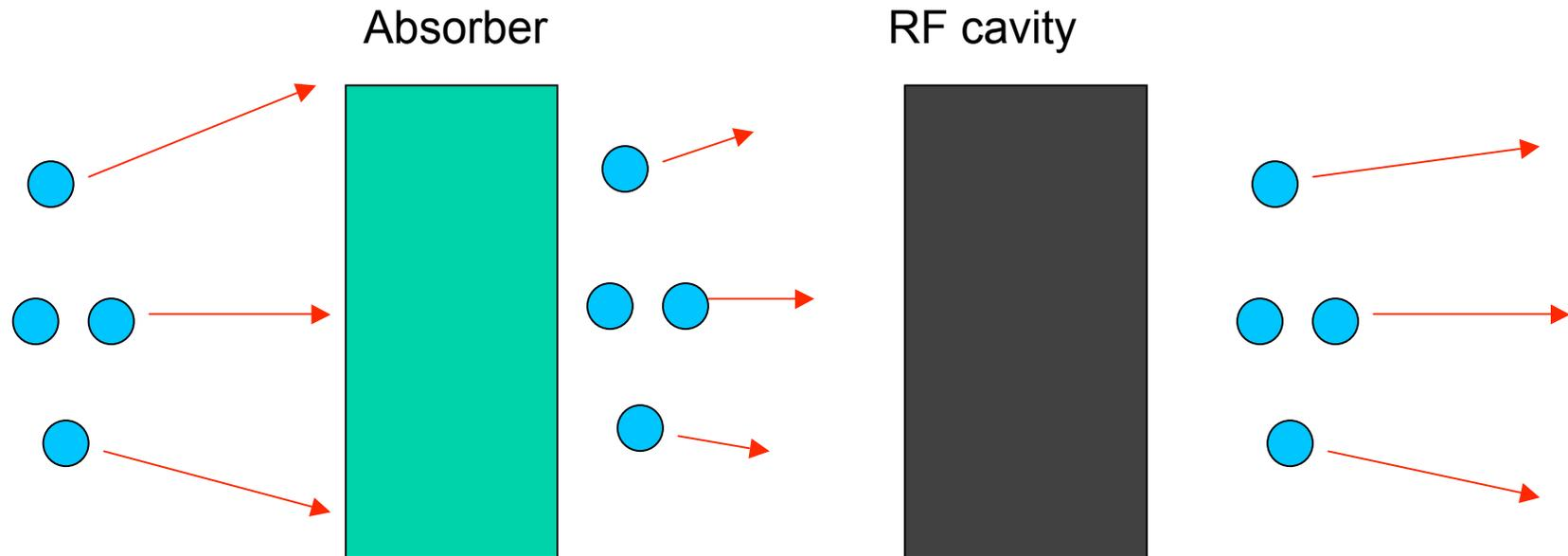
3 D energy loss in Absorber material (Hydrogen)
