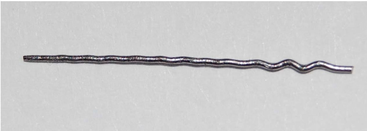
**W5** Tungsten Wire showing "wiggles": 6200 A,  $>2000$  K peak temperature, 5625 pulses.
