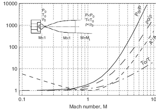
Fig. 9. Isentropic behaviour of a supersonic Laval nozzle with convergent and divergent contours.
