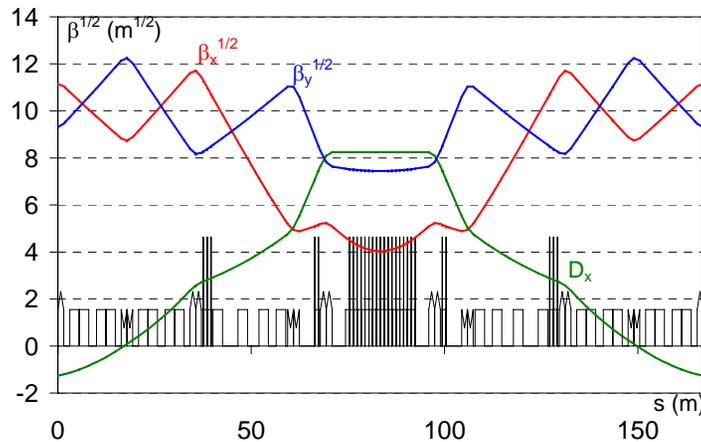
Optical functions in the injection section
